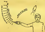
Fig. 5.—Swinging a water bottle in a circle to empty it in the absence of weight. (In reality the liquid coming out would not distribute itself so evenly on the horizontal floor of emptying hall.)
