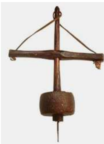
Pump drill: A pump drill is similar to a bow drill, except the thong is tied to the spindle, and then to a crossbar. You wind the thong around the spindle (by turning the spindle by hand to ready it), then push down on the bar to make the drill spin. A flywheel weight keeps the spindle turning, and the thong rewinds itself for the next pump.
