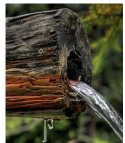
Log pipes are made by drilling out the center of logs with a long auger, and tapering one end, to fit in the next log.
