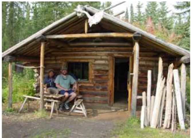
The number, size, and location of cabin doors and windows can be arranged in any manner that you like. Some trapping cabins have been made with no windows, and tiny doors, to keep bears from breaking in.
