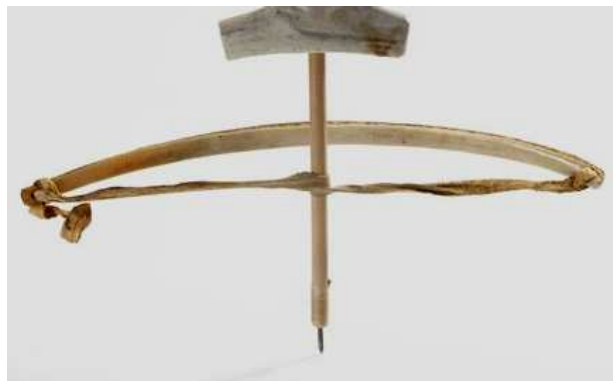
Parts of a Bow Drill: A bow drill consists of a spindle with drill bit, a bow with thong, and a pivot block.
