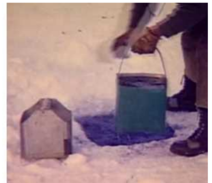
Proenneke made an improvised snow shovel, using poles and part of a metal oil drum. He also attached a large chisel blade to a pole, and used it to cut holes in the lake ice, for collecting water in buckets, and for ice fishing.
