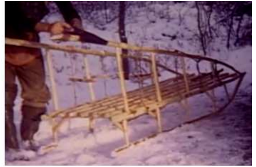
The sled was made from small poles, using the same joinery techniques as used to make the furniture.
