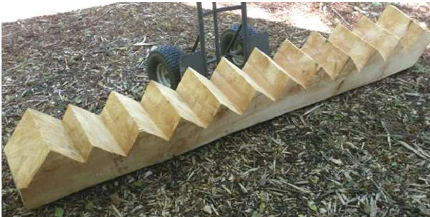
Here is another way to notch a log, to make a log ladder.
