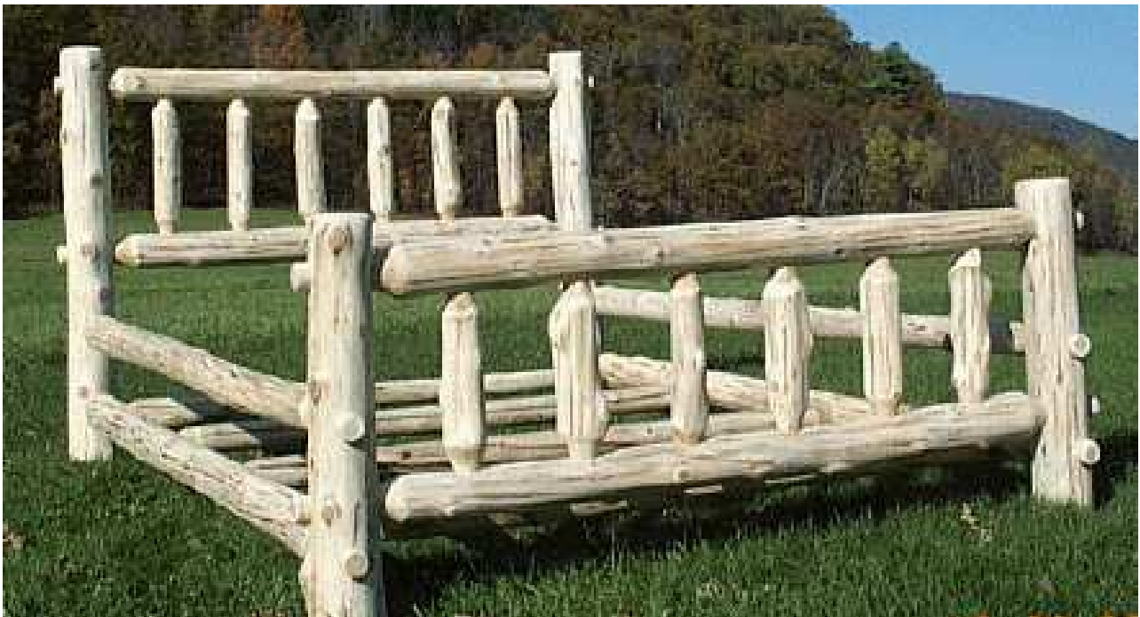
Beds: This bed frame was constructed using the tapered log and drilled hole technique.
