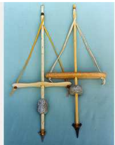
Pump drill: A pump drill is similar to a bow drill, except the thong is tied to the spindle, and then to a crossbar. You wind the thong around the spindle (by turning the spindle by hand to ready it), then push down on the bar to make the drill spin. A flywheel weight keeps the spindle turning, and the thong rewinds itself for the next pump.
